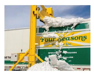
The FleetPlow<sup>™</sup> Model 440T can remove up to 24 inches of snow from a trailer rooftop in less than a minute. This portable snow removal machine can easily be relocated during non-snow months.
