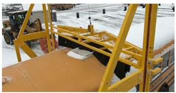
The FleetPlow Model MD-12B can remove up to 12 inches of wet, heavy snow in less than 30 seconds. An up/down pendant control is used to automatically adjust the plow height. There are also more models that can meet operational needs of a wide range of fleet types (from passenger vans to full size buses) and heights (from 75 inches up to 14 feet tall). The machine is portable, which makes it easy to relocate after snow season ends.
