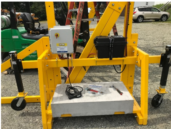
Image 3. Close-Up of Control Box and Battery
